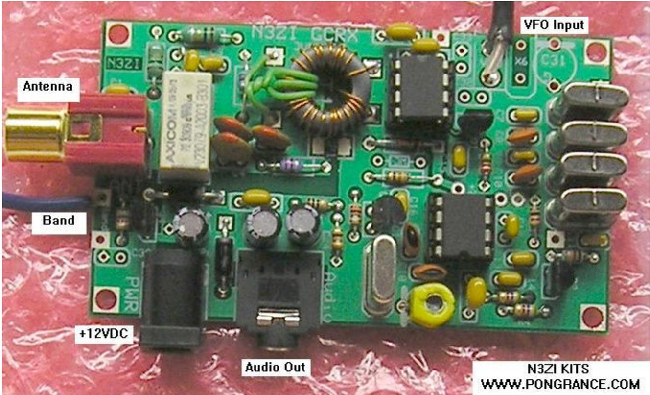
Thank you for purchasing my general coverage receiver kit. You can use the photo above as a guide to assembly. The silk screen on the PCB can also be used as an assembly guide.
