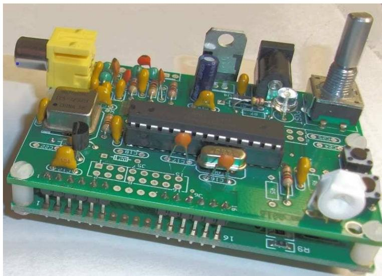
**LCD:** The next step is to connect the LCD. LCDs supplied have a single row of 16 I/O connections, but only 12 of the connections are used, you can skip connection for pins 7-10. R2, 200 ohms, sets the current to the LCD backlight at 7mA. You can decrease this resistor to increase the brightness of your backlight, but do not use a resistor less than 100 ohms (10mA). Kits are shipped with a 4.7K pot for contrast adjustment, which works
