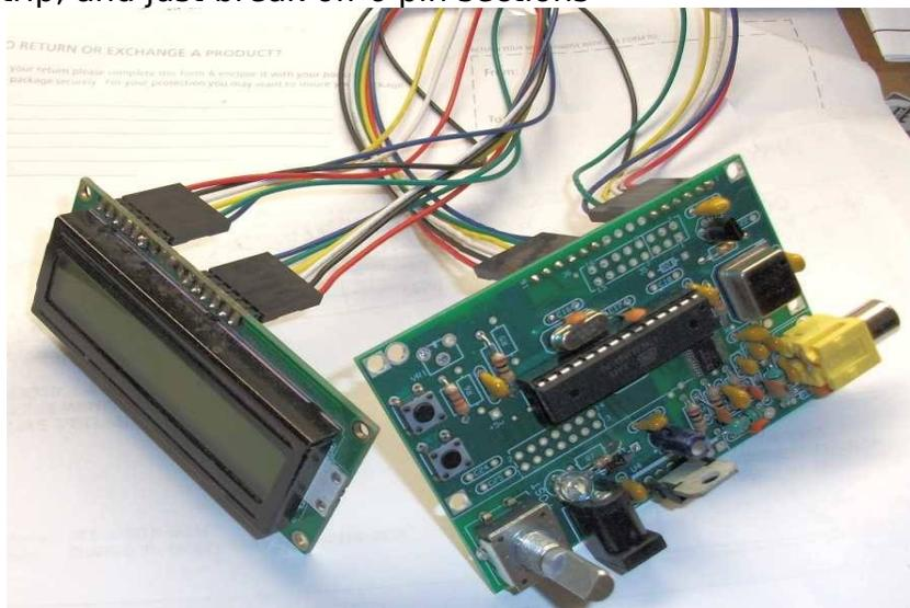
**Final Current check:** With the LCD connected and all parts installed, check and record the current draw, it should be less than 100mA. No parts should be getting hot, except the 80MHz oscillator can may get slightly warm but not hot. The 7805 may get slightly warm, but not hot. If the power on self test LED is working properly, but the LCD is not on check the bias voltage (LCD Pin 3) and wiring to the LCD.
