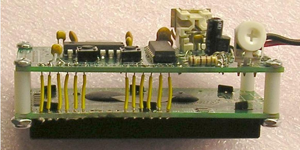
This photo is shown to illustrate with connection to the LCD, the PCB in the above photo shows some additional parts not included in your kit.
