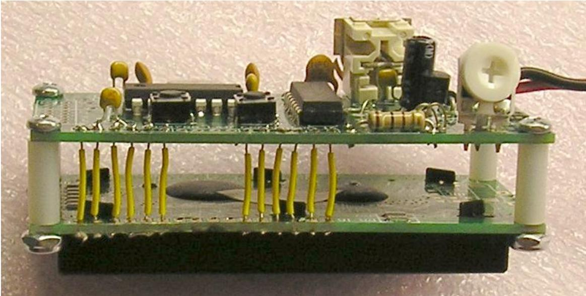
If using the 10K pot, adjust VR1 for 1.2v on LCD Pin 3 (with the LCD connected). The fixed 3.3K resistor will fix this voltage to approx 1.2V.
