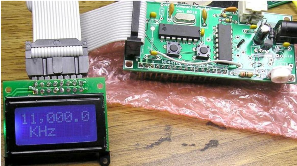
Shown above is the Kit configured for a LCD with a 2 row connector. Note extra jumper, gray wire for backlight. I do not stock these smaller LCDs but they are readily available on ebay.
