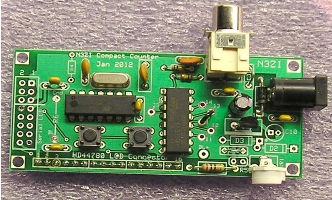
Kit properly assembled and configured for Backlit LCD
