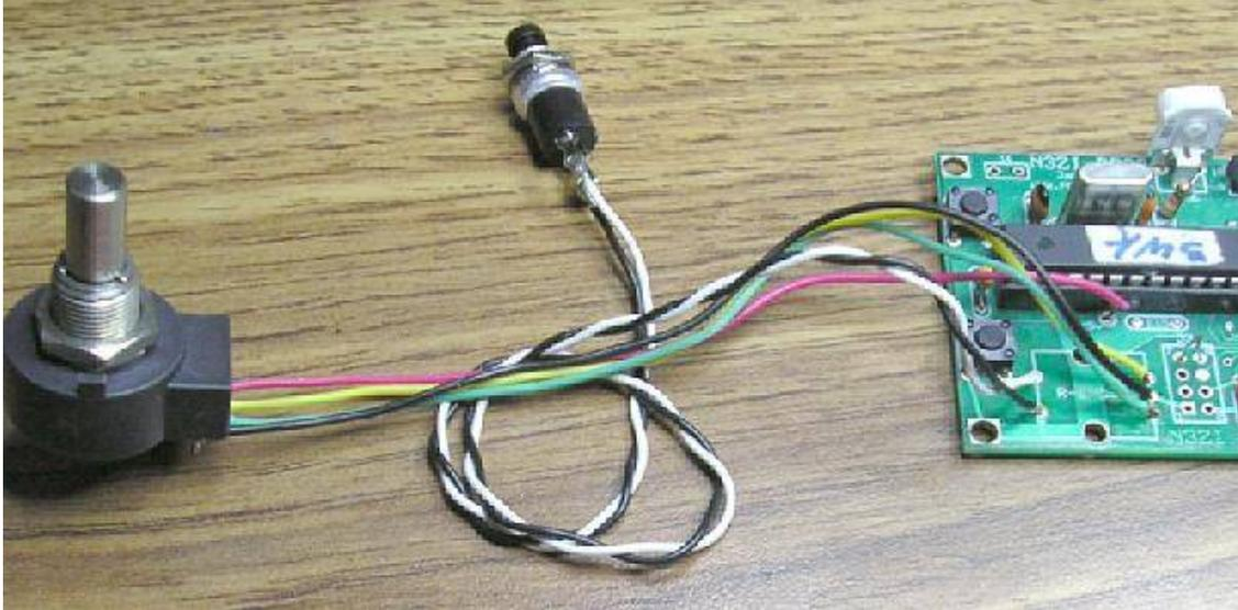
Most Optical Encoders have 4 pins on the back, labeled: + A B -
