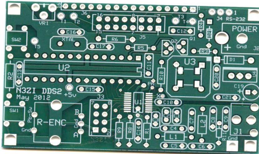
Start by soldering in the power supply components. D1, U4, C19, C20, C21 The PCB is laid out to accept a 2.1mm power connector, but it isn't really needed. This is a 2.1 mm coaxial power connector, +12v inside, ground outside. These connectors usually have 3 pins, there is no PCB hole for the side pin, just break it off. If you don't have a power connector, just solder your power wires directly into the PCB holes. Double check the polarity on D1, C19, and the orientation of U4.
