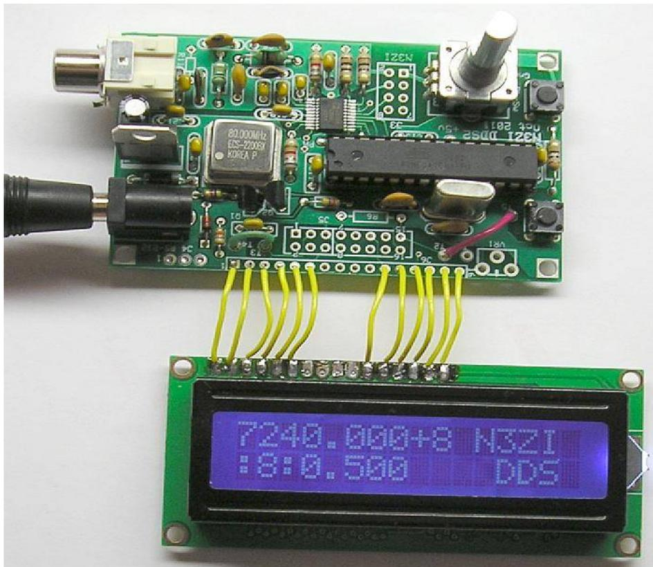
Some displays of this type may have only 14 pins. In this case you would skip pins 15 and 16. LCD's with a 8x2 (or 7x2) connector can be connected to J5, use care with orientation, and left right pin swap, which can damage the LCD. Some LCDs have separate Backlight pins which can be wired independently to backlight power.
