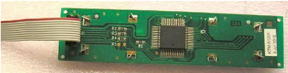
**Photo of back of serial LCD, showing proper orientation of cable [Red Stripe indicates pin 1]**
