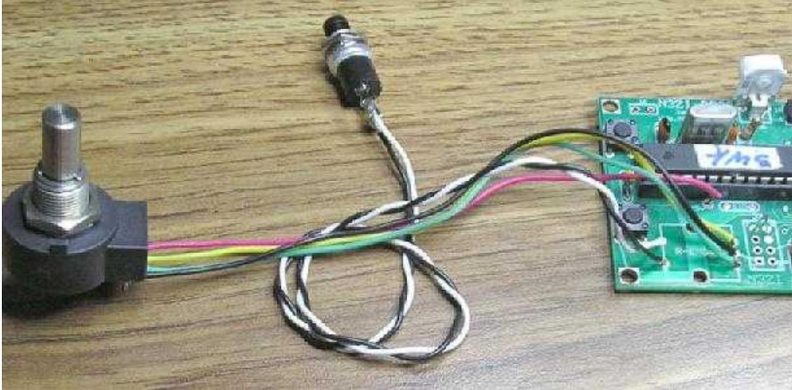
The Optical Encoder has 4 pins on the back, labeled: + A B -
