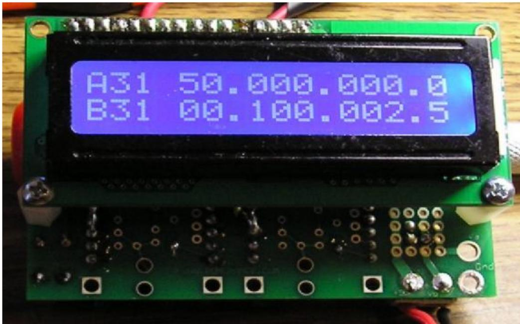
The normal operating range for this device is 100KHz to 40MHz in 1/2 Hz steps. It however can be pushed to DC to 50MHz with some minor changes/accommodations.
