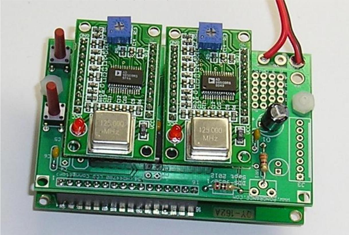
The photo above shows the fully assembled Xtal Bank DDS with 2 DDS modules installed
